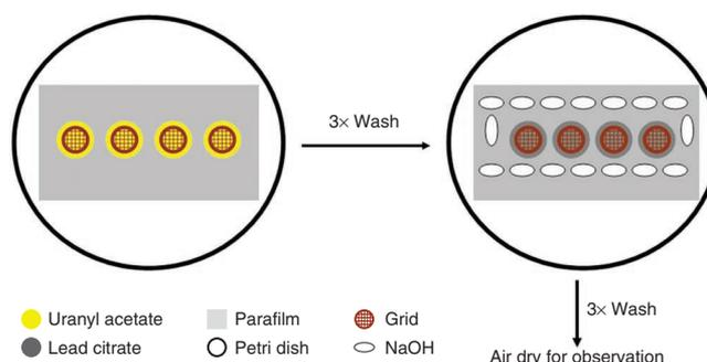
**Figure 4** | Schematic illustrating heavy-metal staining. Note the large number of NaOH pellets (~4 per grid) used with lead staining.
