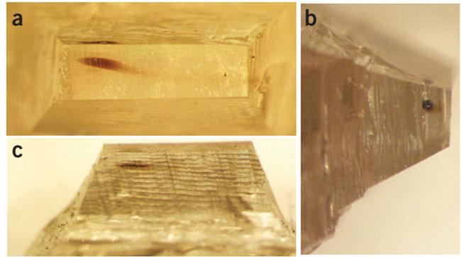
**Figure 3** | An *A. thaliana* root embedded in Spurr's resin after initial trimming. This resin block is trimmed under a dissecting microscope and microtome, using a double-sided razor blade and glass knives. (a–c) View of the block from different sides: top (a), flanking side (b) and front side (c).
