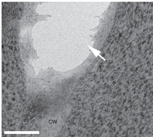
**Figure 6** | An example of section damaged by the electron beam. This kind of instability is often caused by inadequate infiltration. CW, cell wall. Arrow marks the area that was broken under the electron beam. Scale bar, 200 nm.
