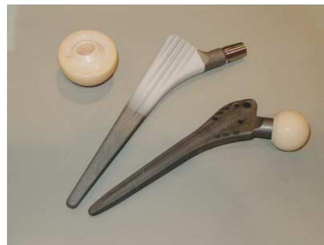
Figure 10. Calcium phosphates in hip endoprostheses: a ceramic ball joint ( $\text{Al}_2\text{O}_3$ ), a calcium-phosphate coated endoprosthesis (“cementless endoprosthesis”) and an uncoated endoprosthesis that must be fixed in place with PMMA bone cement.
